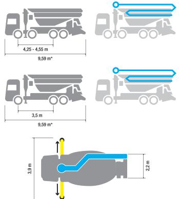
\*Dimensions variable according to the truck assembly
